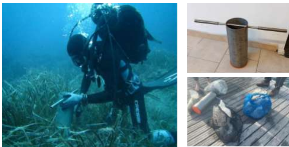
Figure 5.4 Matte sampling using a corer (15 cm diameter, 40 cm length) designed for this study.
