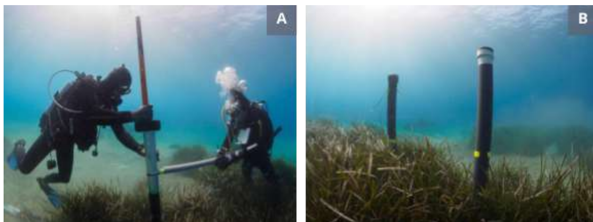
Figure 3.7 (A) Two divers retrieving sediment cores using manual percussion and rotation. (B) Retrieved sediment cores prepared to be transported to the surface.
